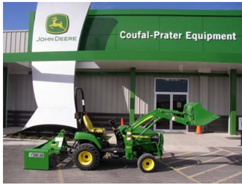
John Deere 2305 4 WD Tractor shown w/JD 200CX Loader and Frontier Box Blade
